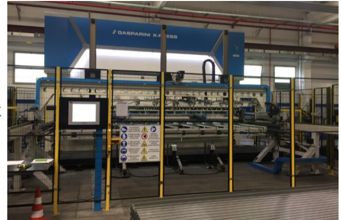
New line for radiant panel
